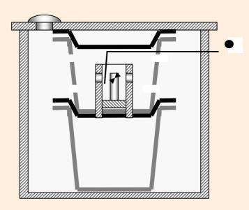
When the reactants are brought into contact, parallel chemical reactions start, resulting in fumigant gas development, being a mixture of phosphine and carbon dioxide
